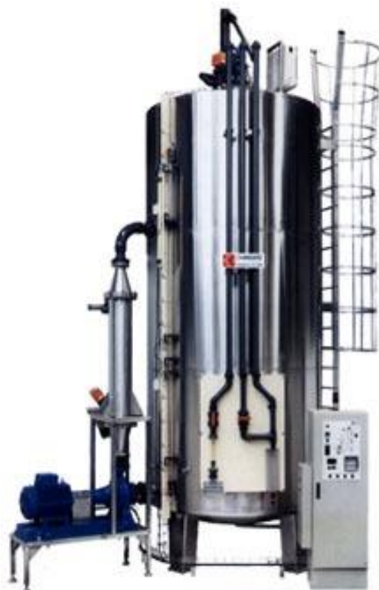
Picture of a bioreactor used to cultivate the micro-organism which produces EPS SEAFILL
